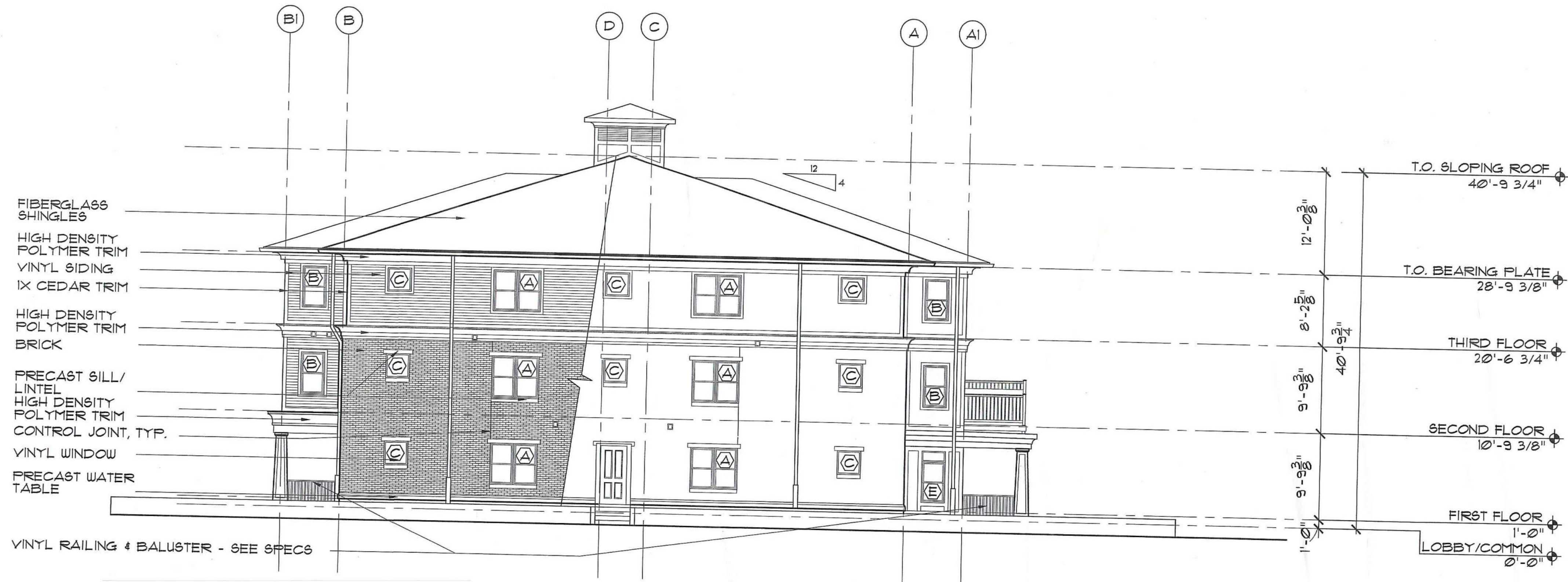
2 NORTH ELEVATION - EDGEWOOD STREET
